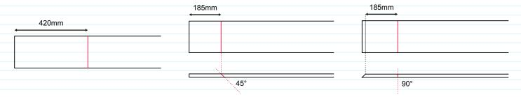
Measure & mark a line 420mm from the end of the pine timber. Clamp securely and cut along the line using a circular saw.
