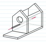
15. Fasten the two side panels to the base and back panel with glue and 32mm brad nails, making sure that the 45° beveled edge matches the angle of the back panel shape.
